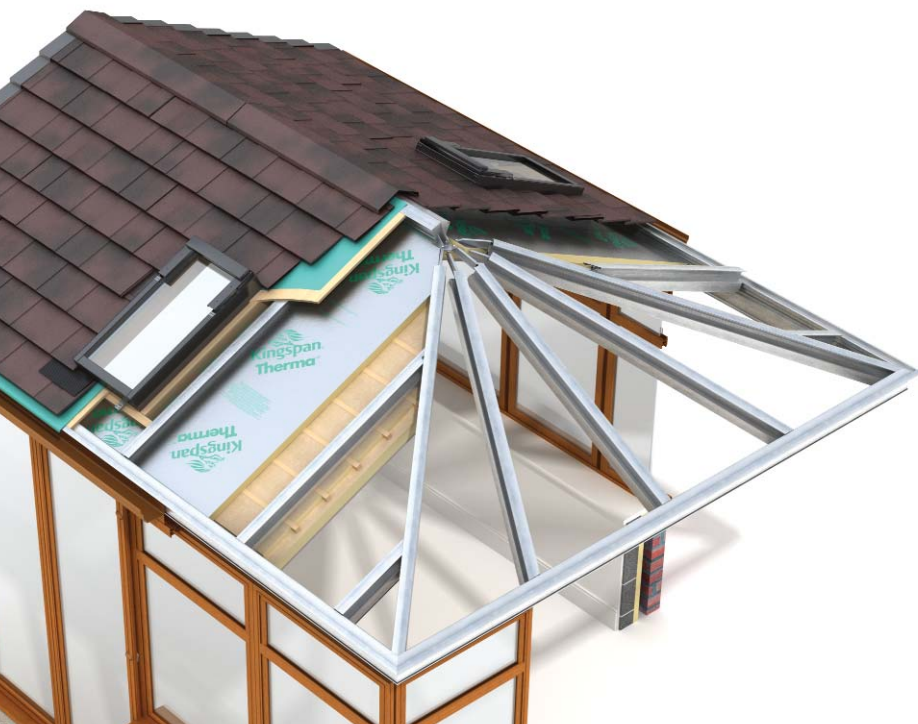
Guardian warm roof construction
